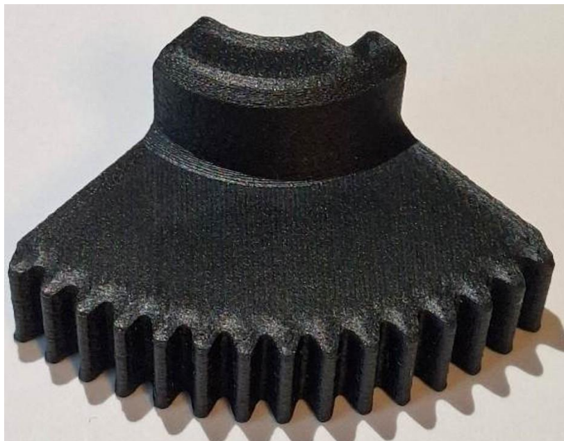
Figure 3: 3D printed sample in the shape of a quarter gear.
