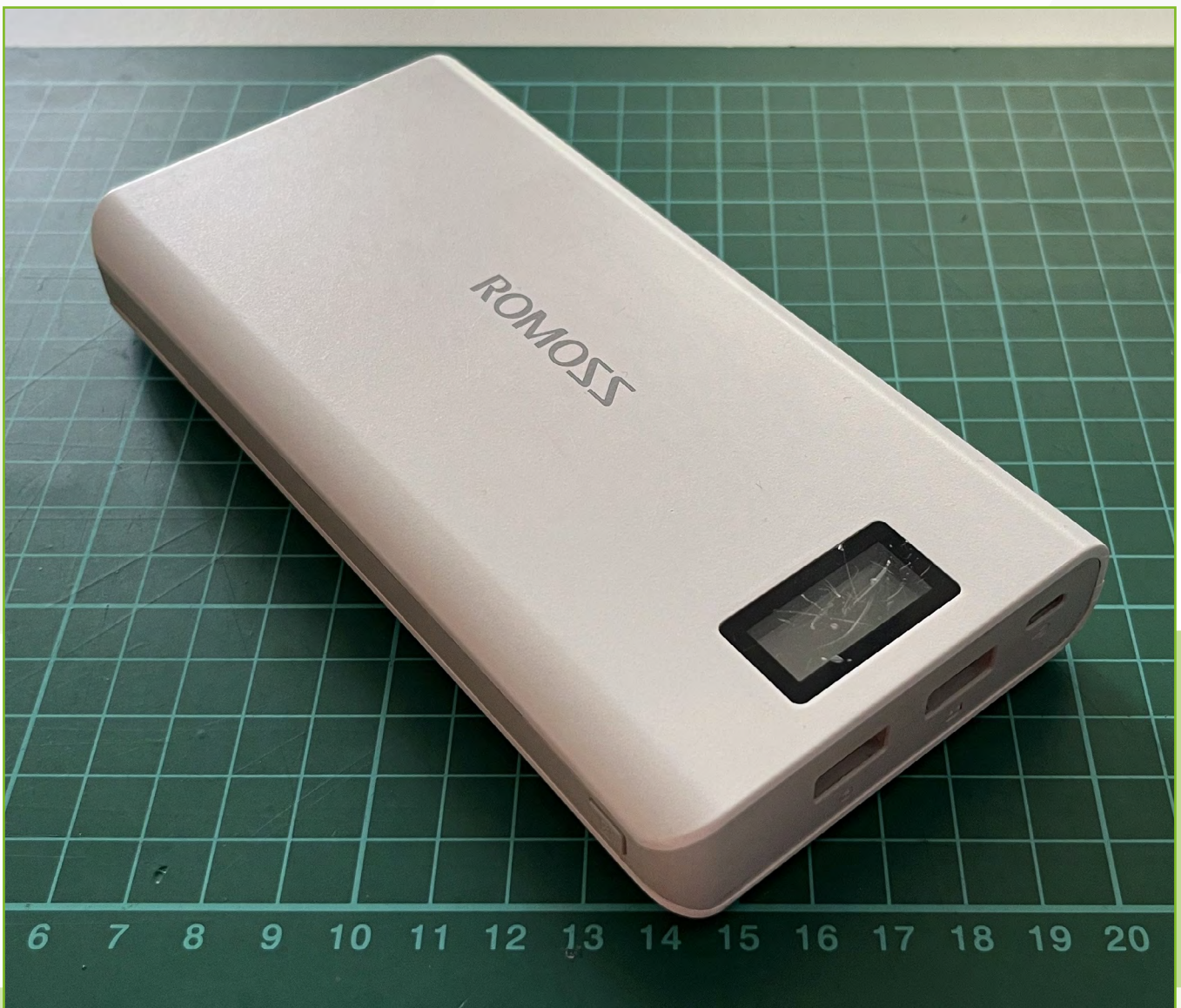
Figure 5: Photo of the analysed power bank. Only its middle part was scanned to achieve better resolution.
