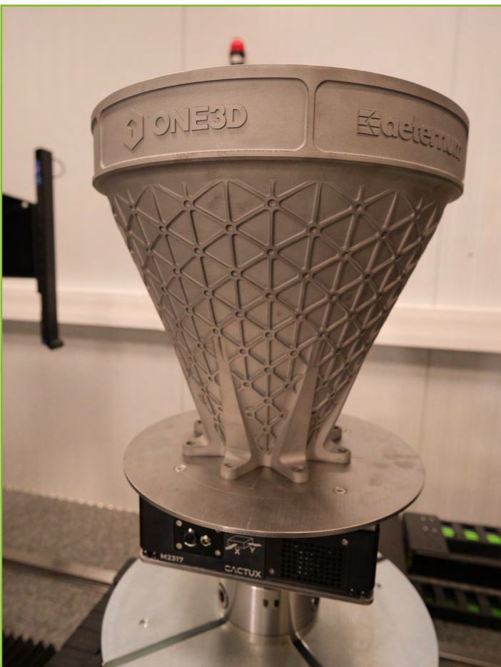
Figure 1: Photo of an additive part inside a CT system.
