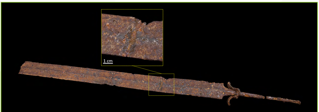
Figure 7: Late Iron Age sword before conservation with traces of pitting corrosion and a secondary defect (marked yellow).
