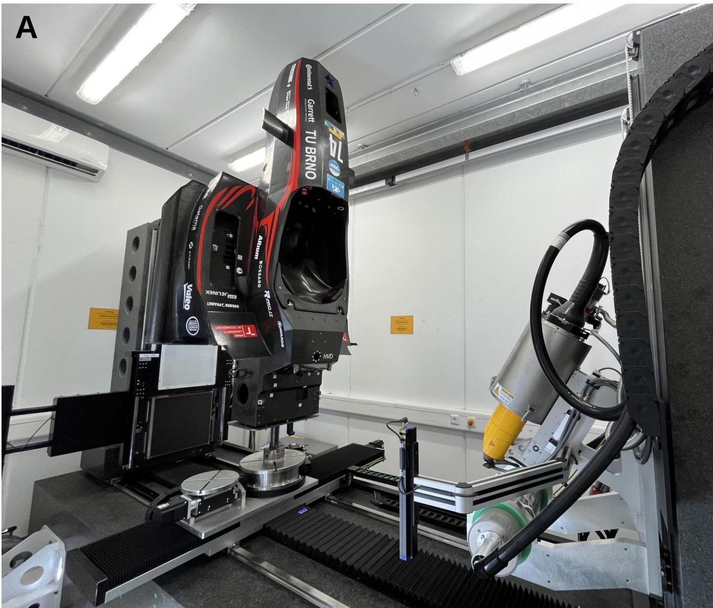
A: illustration of a formula fixation in the CT system B: illustrative cross-section (linear voxel size 80 µm) C: 3D view of monocoque at the front axle suspension point
