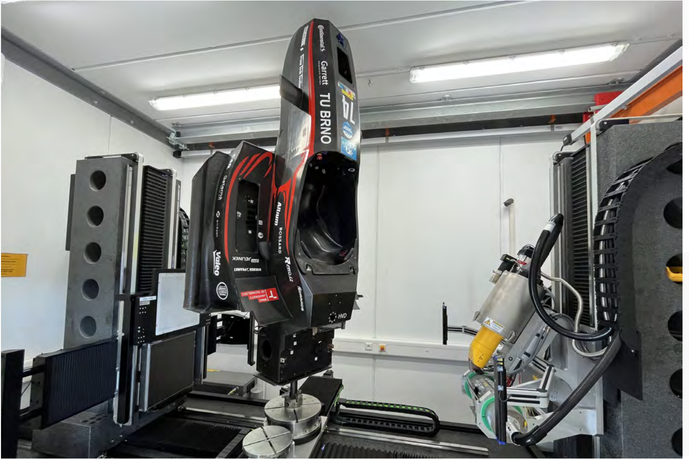
Fig. 5: Picture of the monocoque clamped inside the tomographic system
