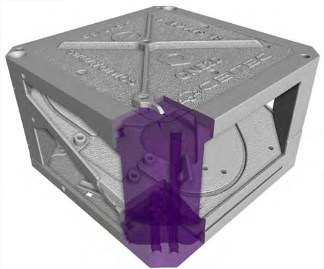
Fig. 2: 3D render of tomographic data of the LLD assembly.
