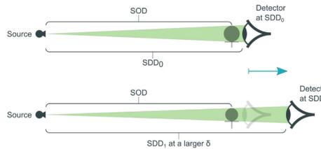
Figure 1: Illustration of the geometry of the Nano3DX. The SOD is large, and only slightly smaller than the SDD. The detector can move along an axis parallel to the X-ray beam, while the sample stays fixed.
