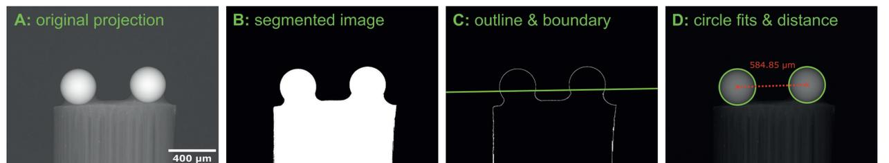
Figure 4: Several major steps of projection processing. A) A radiograph of the phantom. B) Binary mask of segmented phantom. C) Outline of the phantom. Outlines of the two spheres above the green line are used for circle fitting, the rest is discarded. D) Circles are fit on the projections of spheres, and the distance between their centers is calculated
