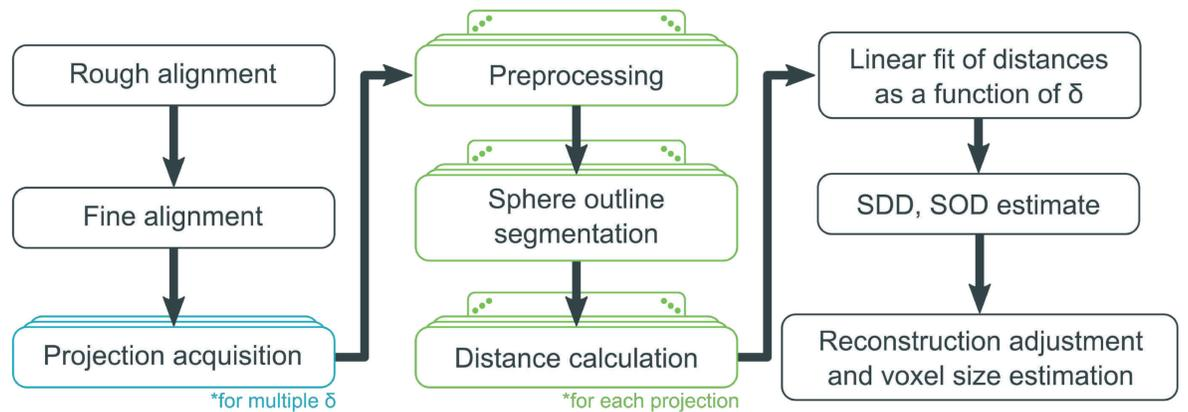
Figure 3: A simplified flowchart of the proposed calibration procedure.
