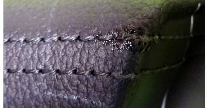
Figure 3: Leak in the armrest.
