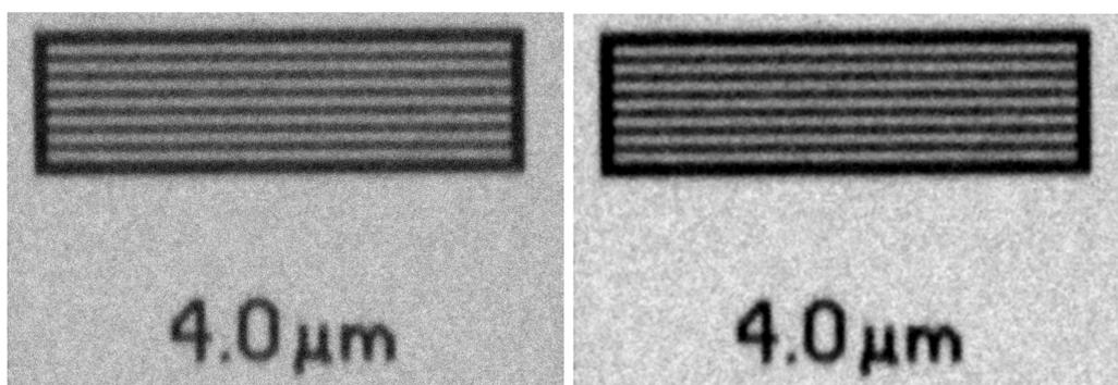
FIG.5. Results of used denoising methodology: left image shows original projection of section of JIMA RT RC-02B bar pattern and right image shows results of used denoising methodology. Random valued impulse noise was reduced using proposed switching median filter and a compound of Read+Shot noise was reduced using NLM [3] algorithm.
