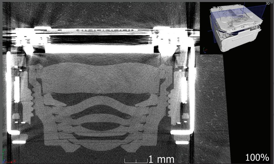
Fig. 3: A tomographic slice in the middle of the camera module from the selected smartphone.
