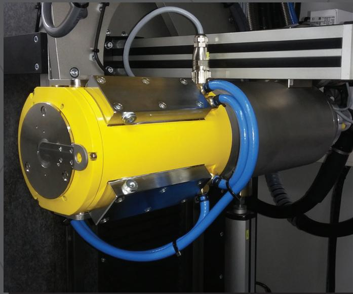
Fig. 6: New nanofocus X-ray tube.
