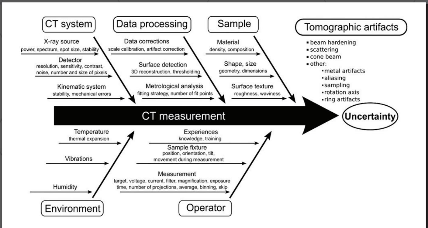
Fig. 4: Diagram shows the influence factors on CT measurement [4].
