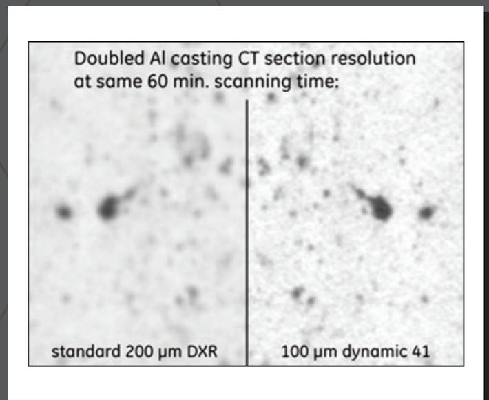
Fig. 5: Tomographic cross section of the aluminium casting, showing the differences between the old and the new detector (picture provided by GE).
