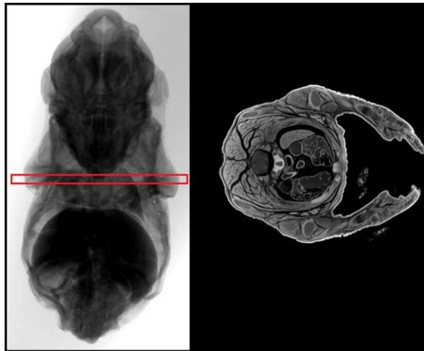
FIG.1. TOMOGRAPHIC RECONSTRUCTION - LEFT IMAGE SHOWS 2D X-RAY PROJECTION AND RED AREA REPRESENTS ONE PIXEL ROW. RIGHT IMAGE IS A CORRESPONDING RECONSTRUCTED SLICE OF MOUSE EMBRYO.
