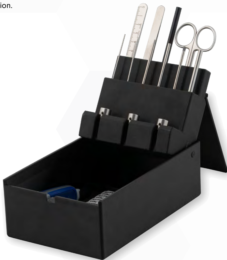
Fig. 10: Essential Toolkit NANO, a complete sample preparation toolkit for submicron CT measurements.
