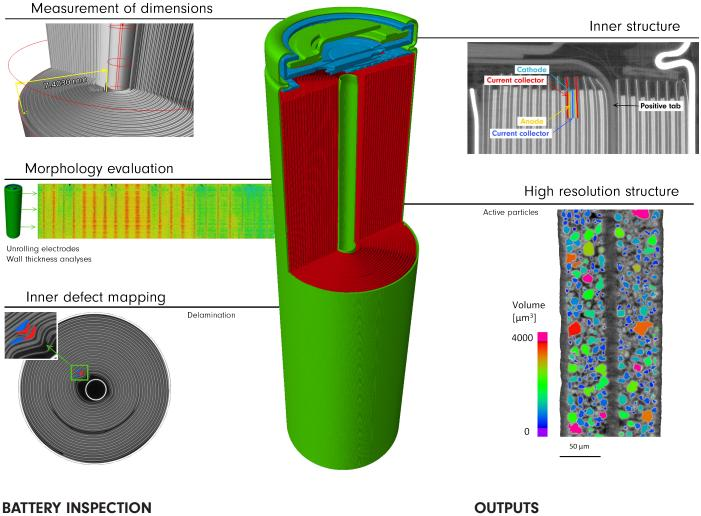
Non-destructive 3D inspection. Defect identification. Electrode investigation. Multiscale imaging. Tracking electrode degradation. Complementary studies. Cross-sections with data viewer. Pictures and videos. STL and STP model. Expert report.
