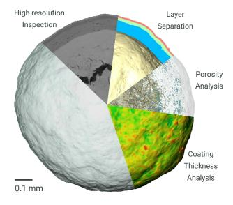
Figure 1: nano3DX particle analysis possibilities.
