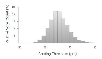
Figure 4: Coating thickness homogeneity analysis—the thickness of the outer coating layer (cellulose acetate layer) of the analyzed particle varied from 50 to 80  $\mu m$ , reflecting low manufacturing quality.
