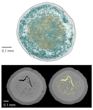
Figure 3: Porosity analysis—in the internal structure of the analyzed particle, a high number of pores were detected, which is reflected by the total porosity of 7.43 percent. Color coding was used according to distance from particle center: Pores in the core layer are yellow and pores in the outer layers are blue.
