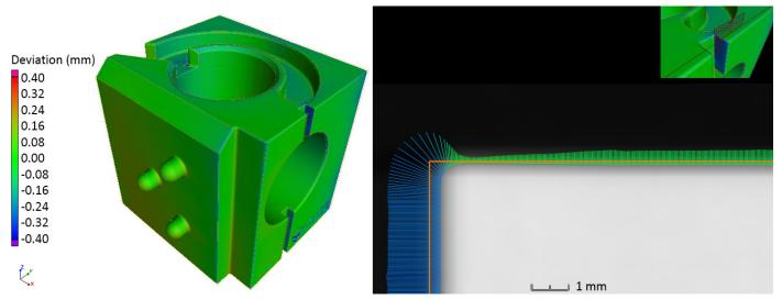
The color map shows the deviations from the surface of the nominal CAD model. The CAD model is marked in orange.
