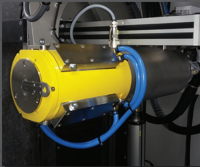
Fig. 6: New nanofocus X-ray tube.
