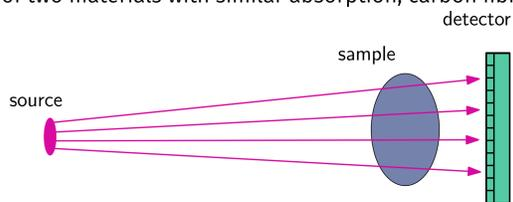
Figure 1: Experimental arrangement of RIGAKU Nano3DX CT device.
