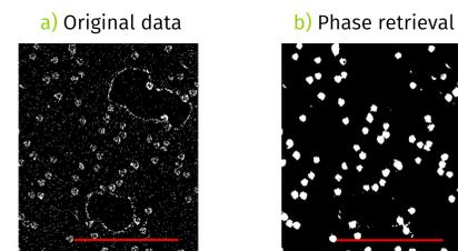
Figure 5: Segmentation of carbon fibres in PE on original data and on data processed with phase retrieval algorithm based on global thresholding according to histogram. Length of the scale bar is 100  $\mu\text{m}$ .
