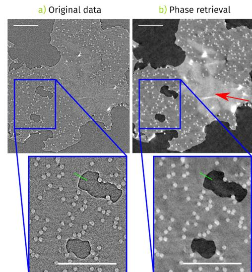
Figure 2: Tomographic section of carbon fibres reinforced PE sample. Length of the scale bar is 100  $\mu\text{m}$ .
